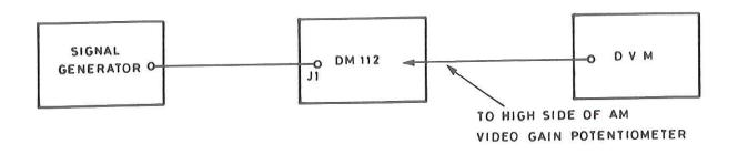
Fig A3 Test set-up: AM sensitivity
