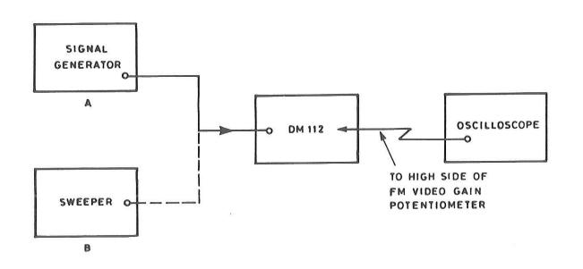
Fig A2 Test set-up: FM discriminator sensitivity
