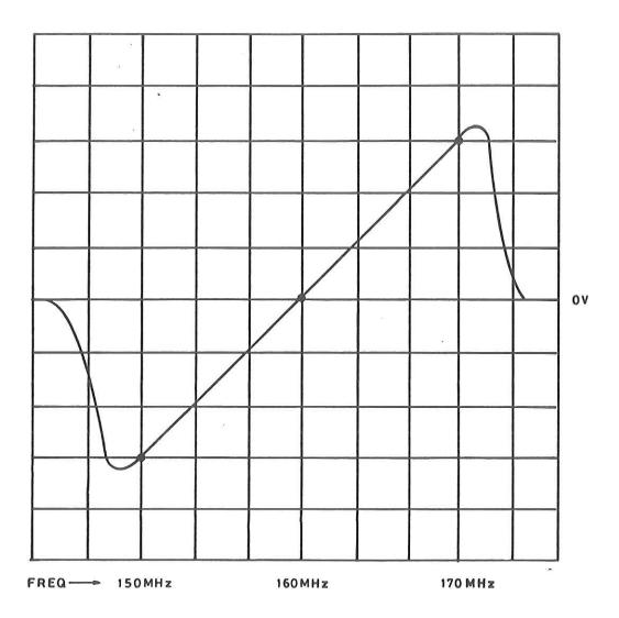
Fig 10 'S' curve 20 MHz bandwidth
