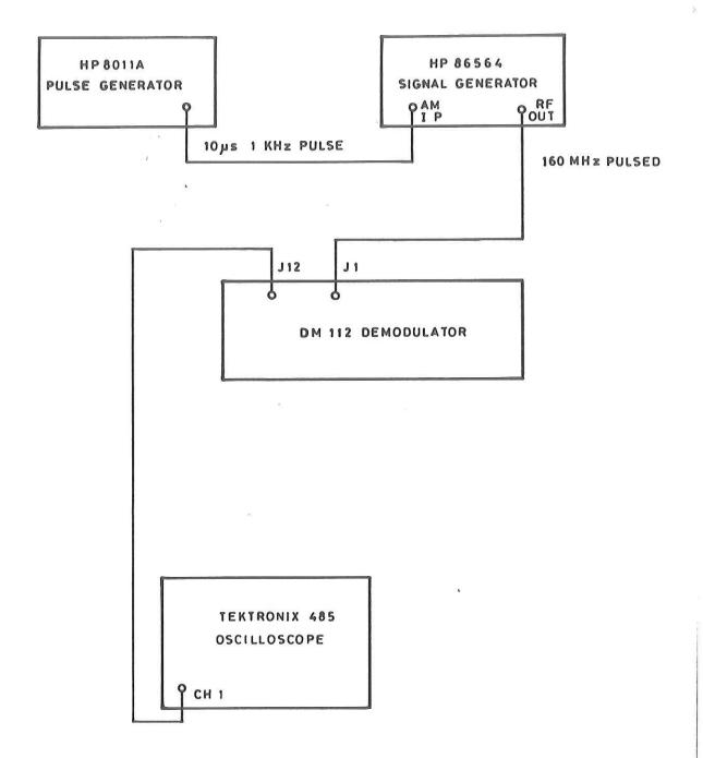
Fig 11 Test set-up for IF and video tests
