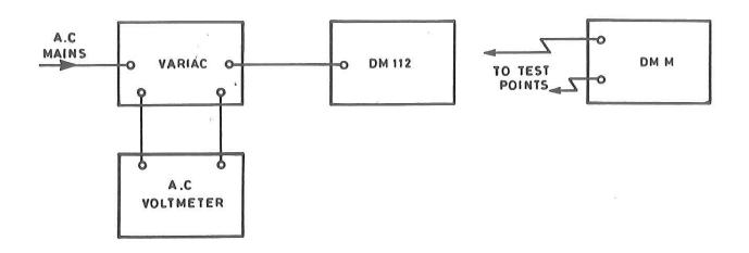
Fig A1 Test set-up: power supplies
