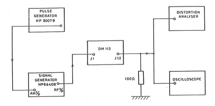
Fig A7 Test set-up: pulse stability
