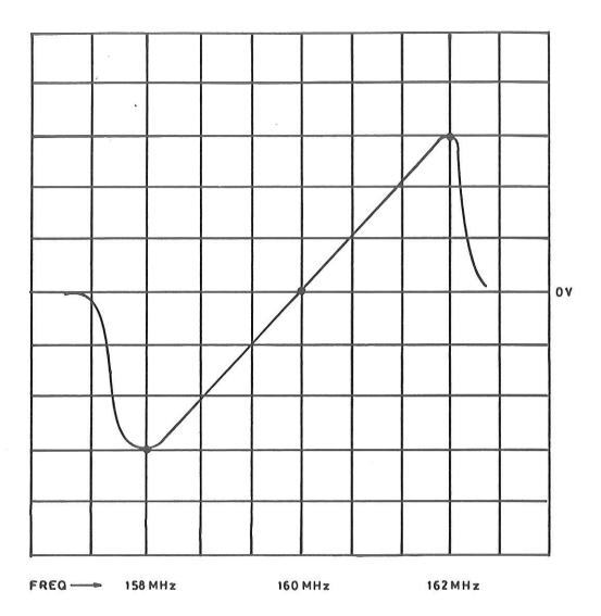
Fig 9 'S'curve 4MHz bandwidth
