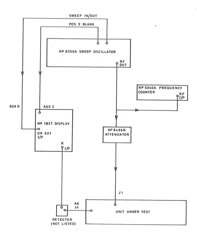
Fig 1 Test set up for AM alignment
