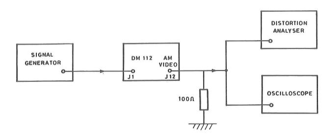
Fig A5 Test set-up: AM/AGC video output
