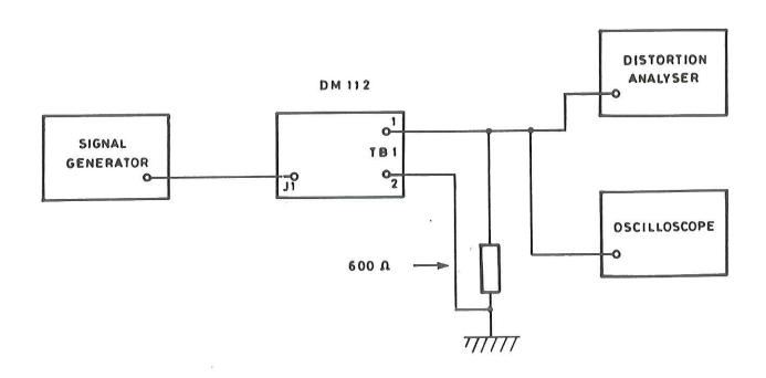
Fig A4 Test set-up: audio output level
