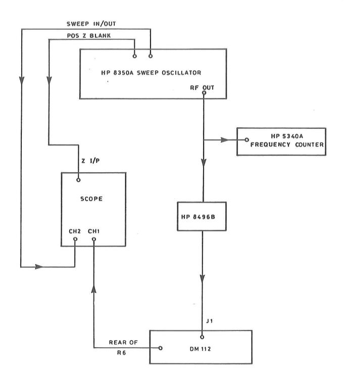
Fig 7 Test set-up for discriminator 'S' curve
