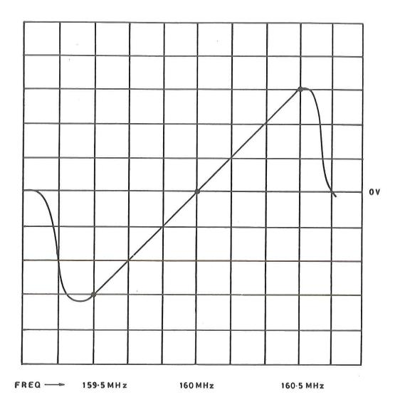
Fig 8 'S'curve 1MHz bandwidth
