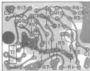
Figure 5-15. Part 17452-2 IF Output (A2A3), Location of Components
