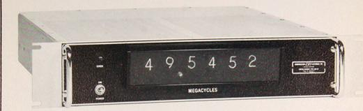
The Type DRO-50 Counter has been designed as a companion unit for the Hammarlund SP-600-( ) receiver which tunes from 0.54 to 54 mc. The counter provides a direct digital display of the frequency to which the receiver is tuned by counting the local oscillator frequency and automatically subtracting the intermediate frequency in use.
