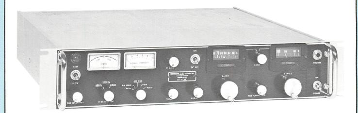
The CEI Type 977 Receiver is designed for the reception of AM, FM, CW, and pulse signals in the VHF frequency range of 30-300 MHz. It is an all solid-state receiver utilizing dual-gate MOS field-effect transistors in all critical stages in both the RF tuners and IF amplifiers. This, combined with CEI's "know how" in receiver design results in a unit having maximum sensitivity combined with a very large dynamic range and low cross-modulation characteristics.
