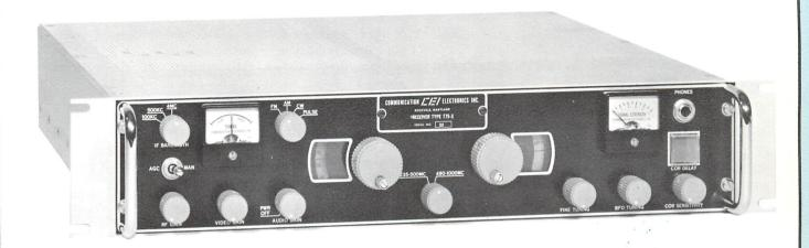
The Type 775-3 Receiver is designed for the reception of AM, FM, CW, and pulse signals in the UHF frequency range of 235 to 1000 MHz. Modern components and techniques have been used to obtain maximum performance and retain the advantages of small size and low power consumption. A carrier operated relay (COR) circuit is standard on the 775-3.
