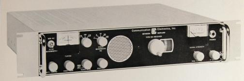
The CEI Type 501 Receiver is a compact, highly stable unit designed for the reception of AM, FM, and CW signals in the frequency range of 54 to 260 megacycles. The unit is useful as a general purpose laboratory receiver, and in telemetry and monitoring applications.
