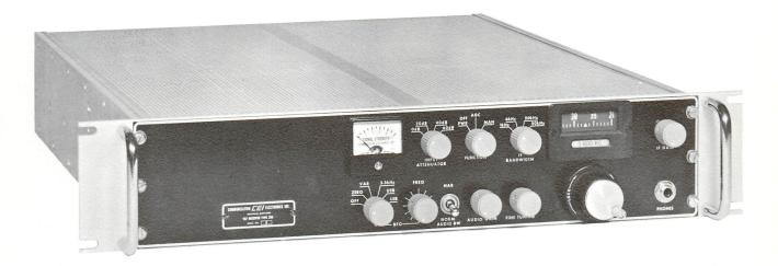
The CEI Type 355 Receiver is a wideband unit designed for RFI and EMI detection in the frequency range of 1 kHz to 600 kHz. The receiver covers this frequency range in a single band. Selectable IF bandwidths of 1 kHz, 6 kHz, 20 kHz, or 50 kHz have been provided to facilitate the detection of both wideband and narrowband signals. The frequency response of the audio amplifier is extended to 50 kHz to match the widest IF bandwidth for use with an impulse generator.
